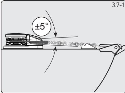
1. Lead from the roller should be fed horizontally back to the top of the gypsy and along its centre line within  $\pm 5^\circ$ .
