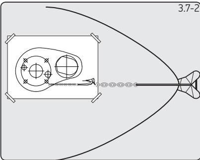
2. Using your template and after you have checked all the above and below deck requirements cut the following holes.
