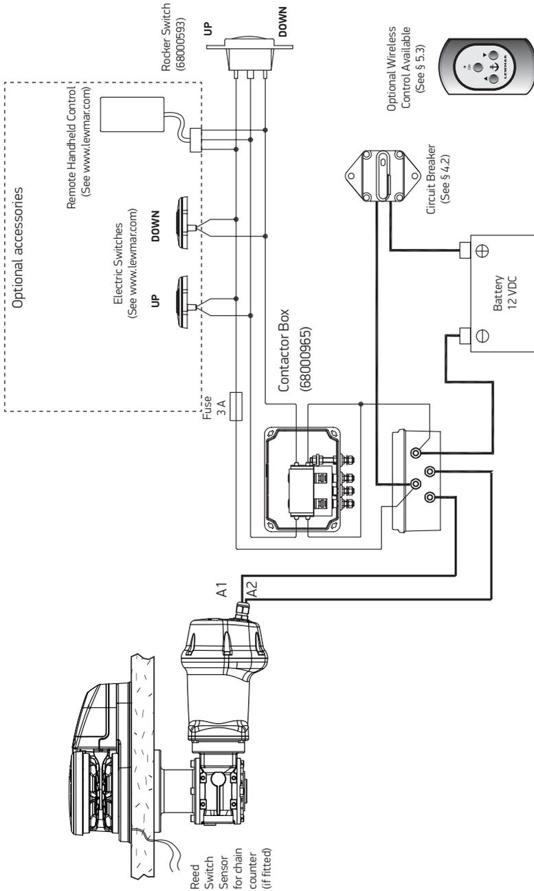
**4.7 VX1l - Wiring diagram if a contactor box (Part No 68000965) is used**
