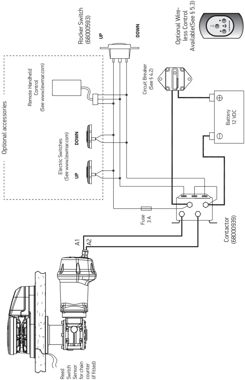
**4.5 VX1 - Wiring diagram if a contactor box (Part No 68000965) is used**
