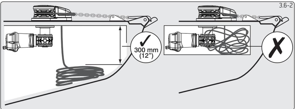
2. There must be sufficient vertical fall for the chain or rope when hauling in.
