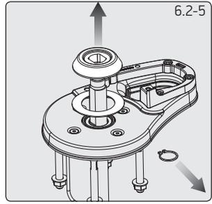
Assemble the new gypsy in reverse order, note that the part number engraved on the stripper ring should face upwards.
