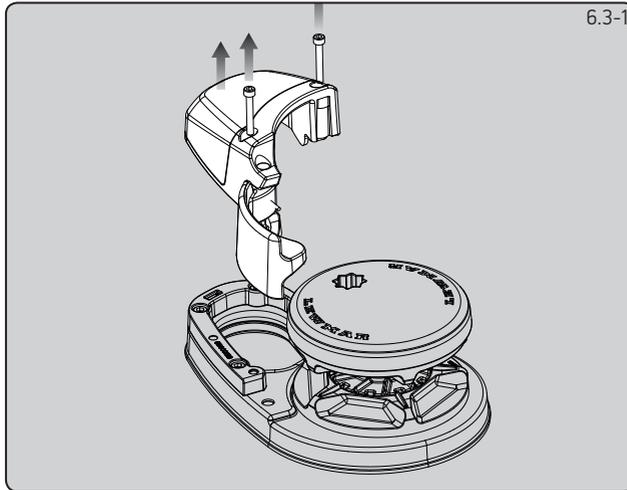
⚠ WARNING! Isolate the windlass using circuit breaker/isolator.
