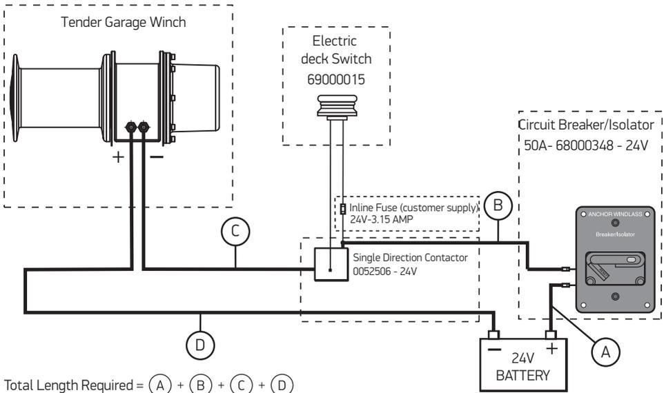
Only one type of switch is required, though more than one may be fitted.
