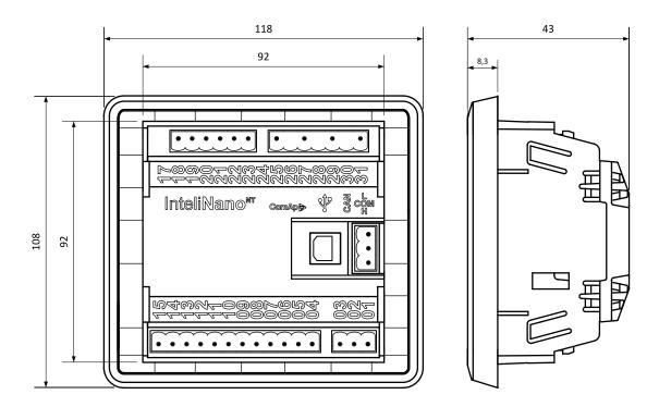
**Note:** The controller is to be mounted into panel doors as a standalone unit using provided fixing clips. The requested cut-out size is  $94 \times 94$  mm. Use the screw holders delivered with the controller to fix the controller into the door.
