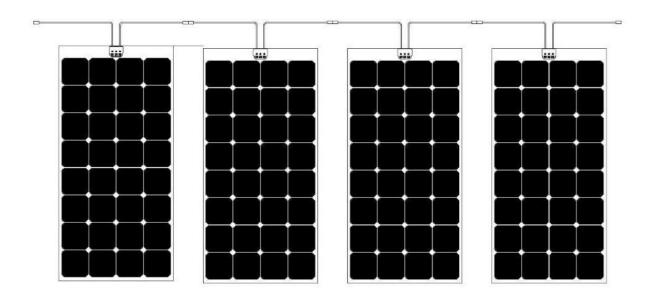
Modules of the same type can be always connected in series. The connection in series between different types of modules can be done only after Enecom technician's authorization.
