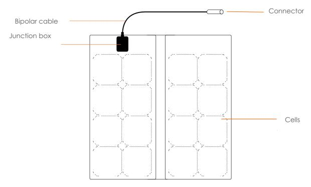
In HFp modules the junction box is positioned on the back surface.
