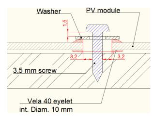
During mounting, avoid applying pressure on the cells or overbidding the panel.
