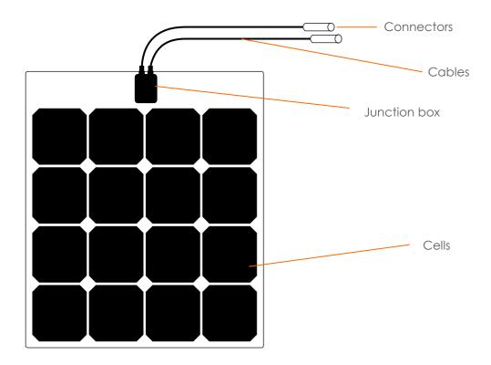
The junction box, at the request of the customer, can be placed on the back surface.
