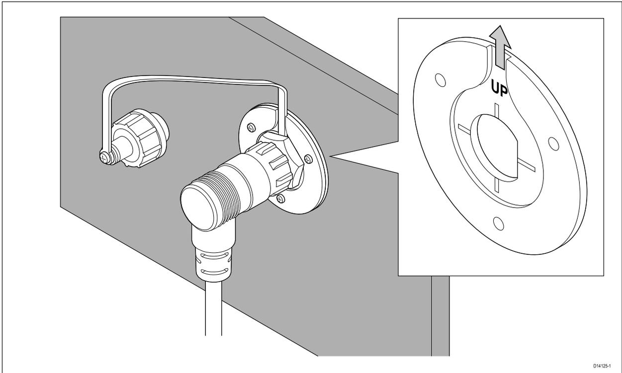
To ensure that the handset's connector points down when connected, orientate the mounting plate so that the lanyard groove is pointing straight up.
