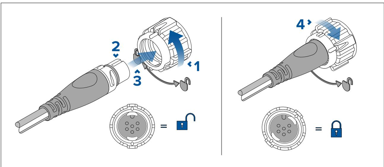
1. Rotate your product's SeaTalkng<sup>®</sup> connector locking collar counter clockwise, so that the connector is in the unlocked position.
