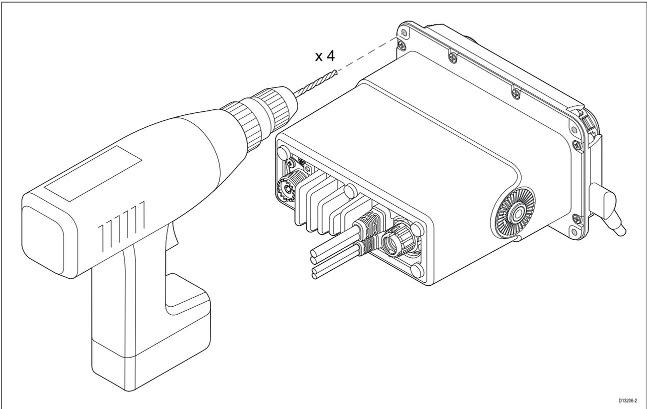
1. Using a drill and a 4 mm (5/32) drill bit, drill out the 4 mounting holes.
