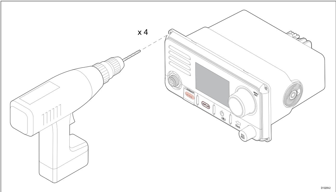
1. Using a drill and a 4 mm (5/32) drill bit, drill out the 4 mounting holes.
