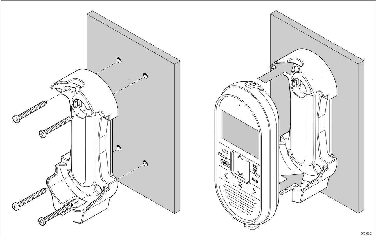
1. Check the selected location for the mounting holster, a clear flat area is required, with sufficient space around it to place and remove the handset.
