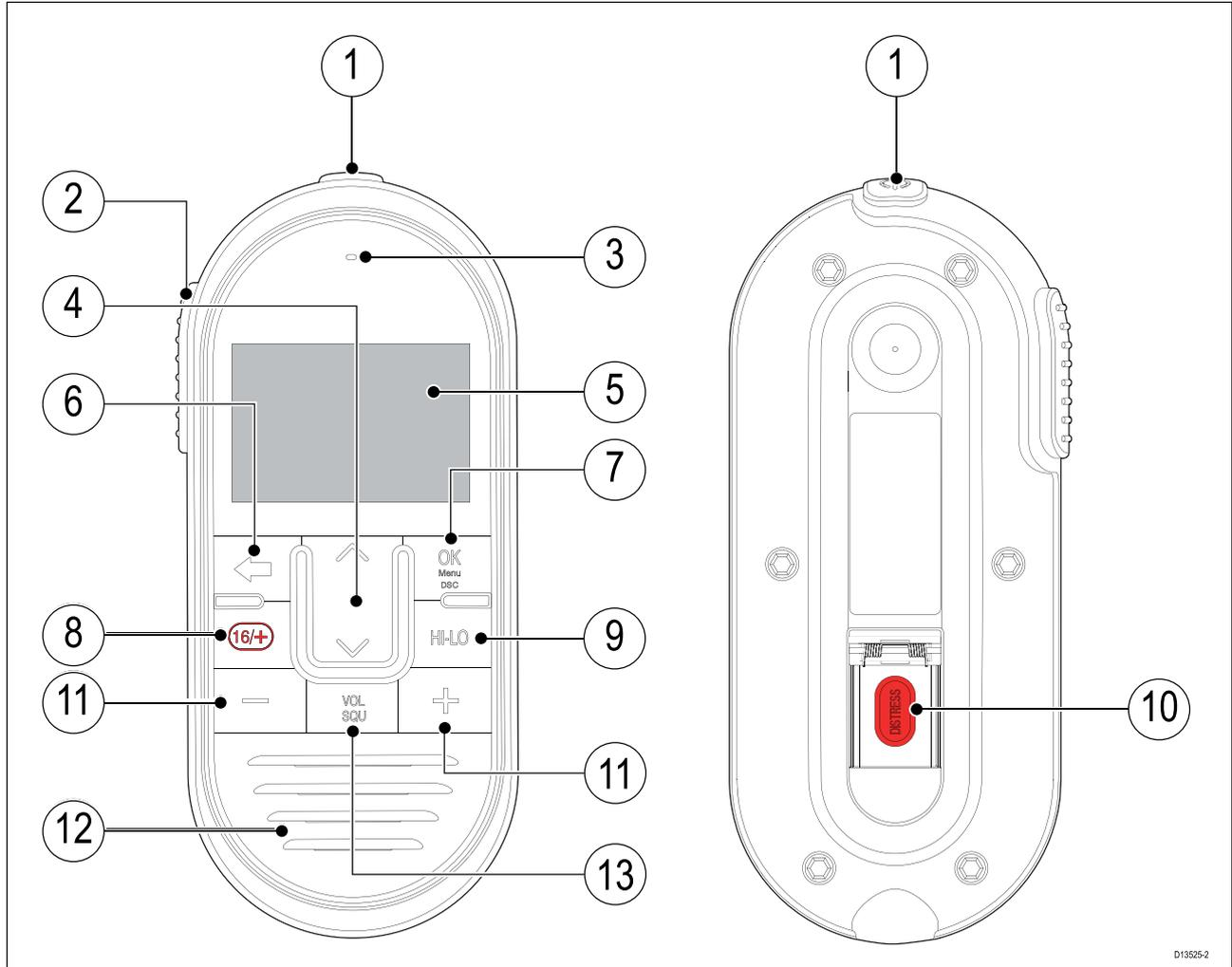
1. **Power** — Press to power the handset on. Press and hold for 3 seconds to power the handset off. Momentary press to access the shortcut list.
