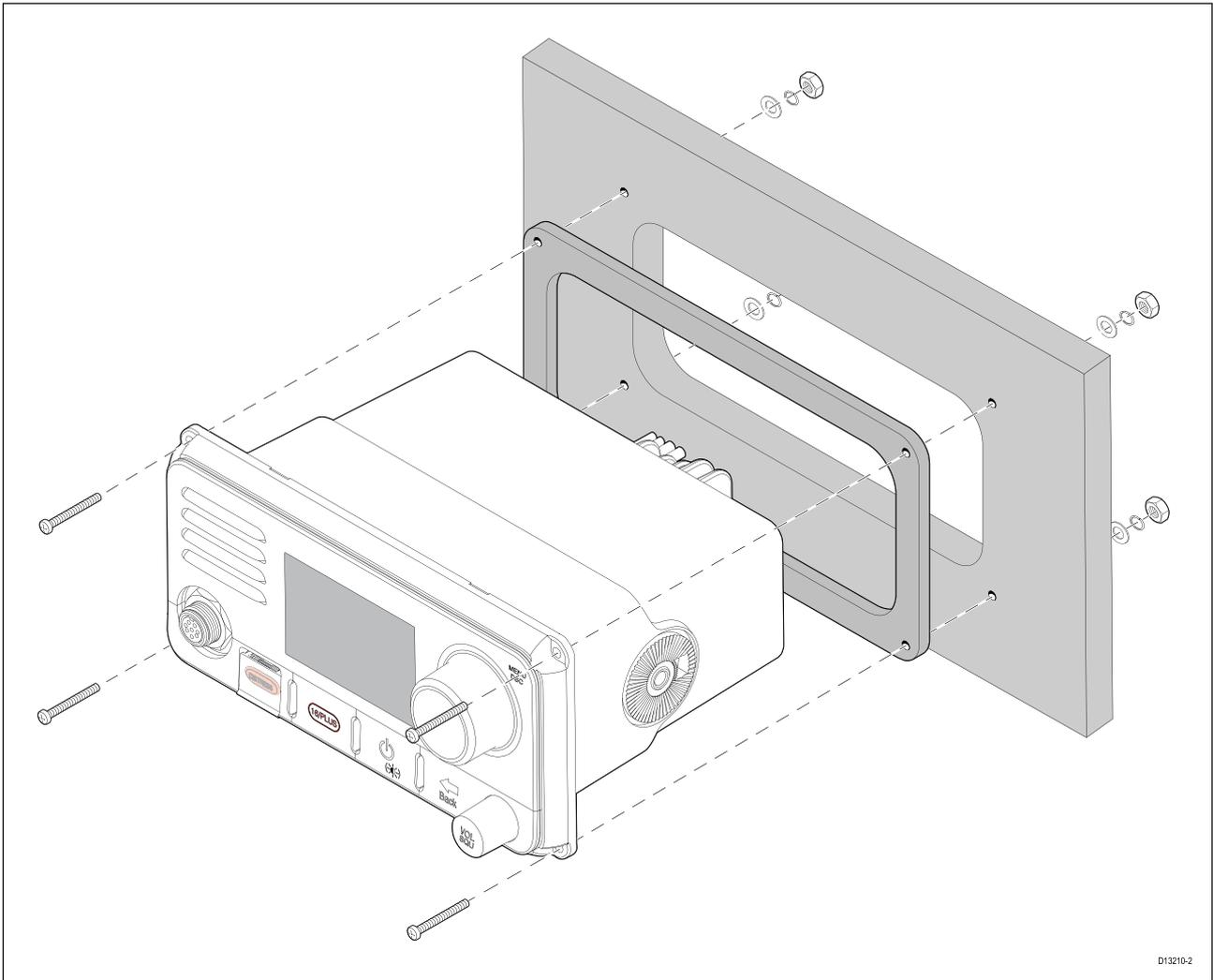
1. Check the selected location for the unit. A clear, flat area with suitable clearance behind the panel is required.
