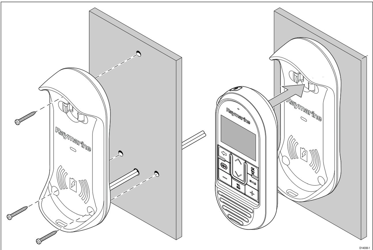
1. Using the supplied mounting template mark the location of the mounting holes and if required, the cable hole.
