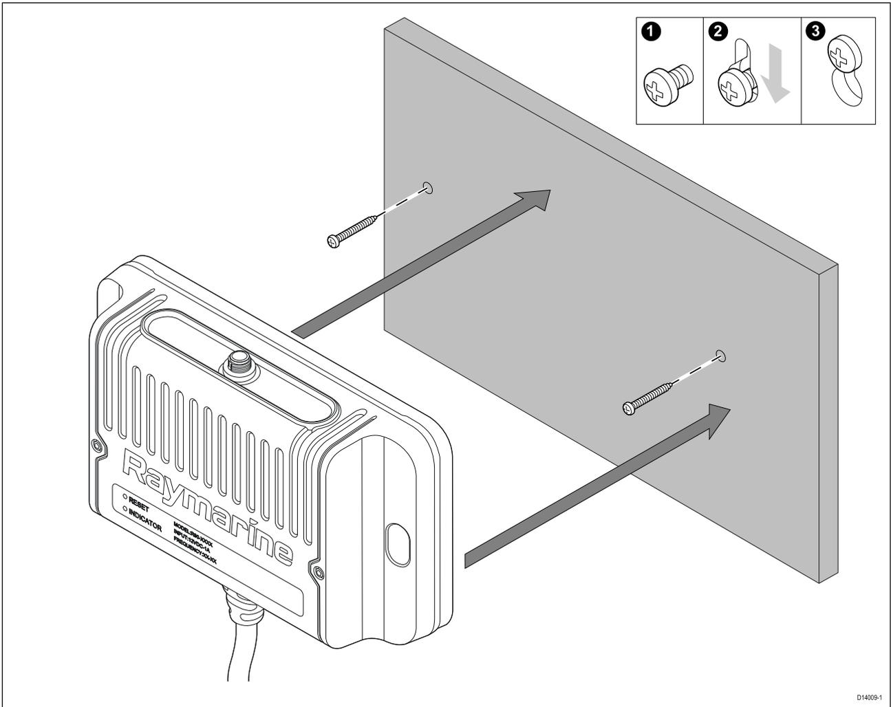
1. Using the supplied mounting template, mark the location of the fixing holes on the mounting surface.
