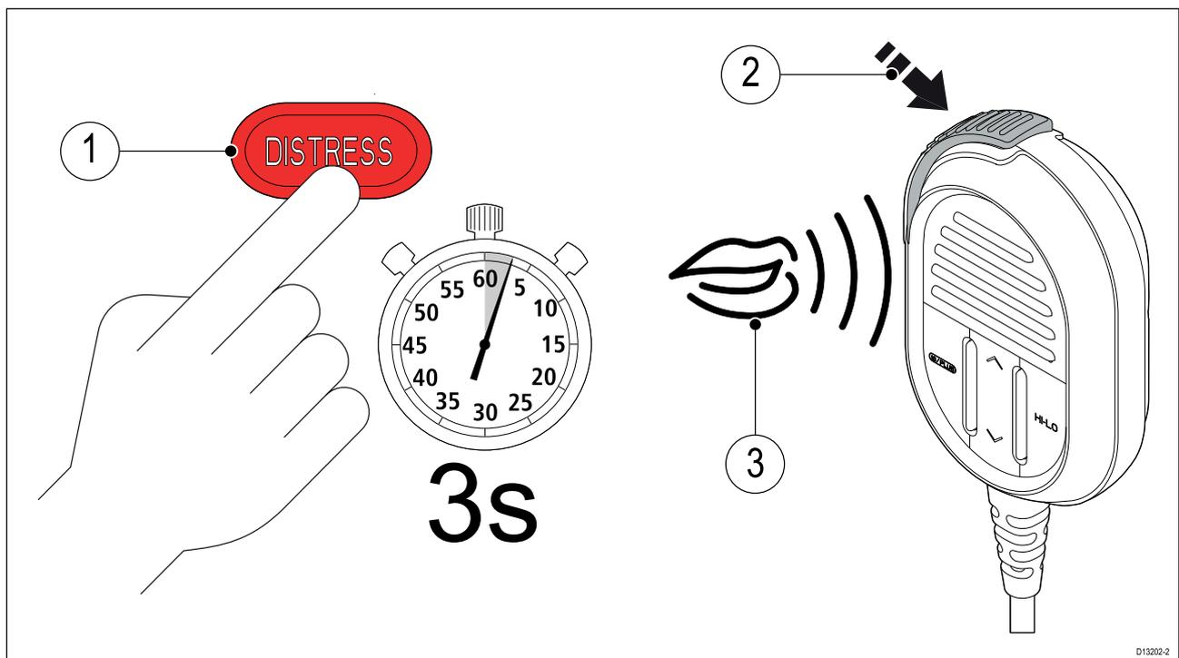
1. Press and hold the **DISTRESS** button for 3 seconds.
