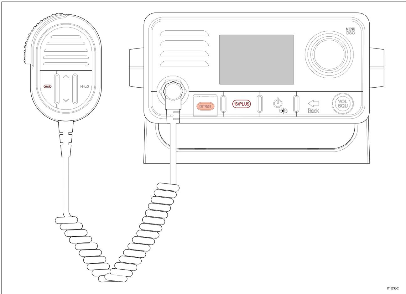
The Fistmic can be connected directly to the front connector on your Radio.
