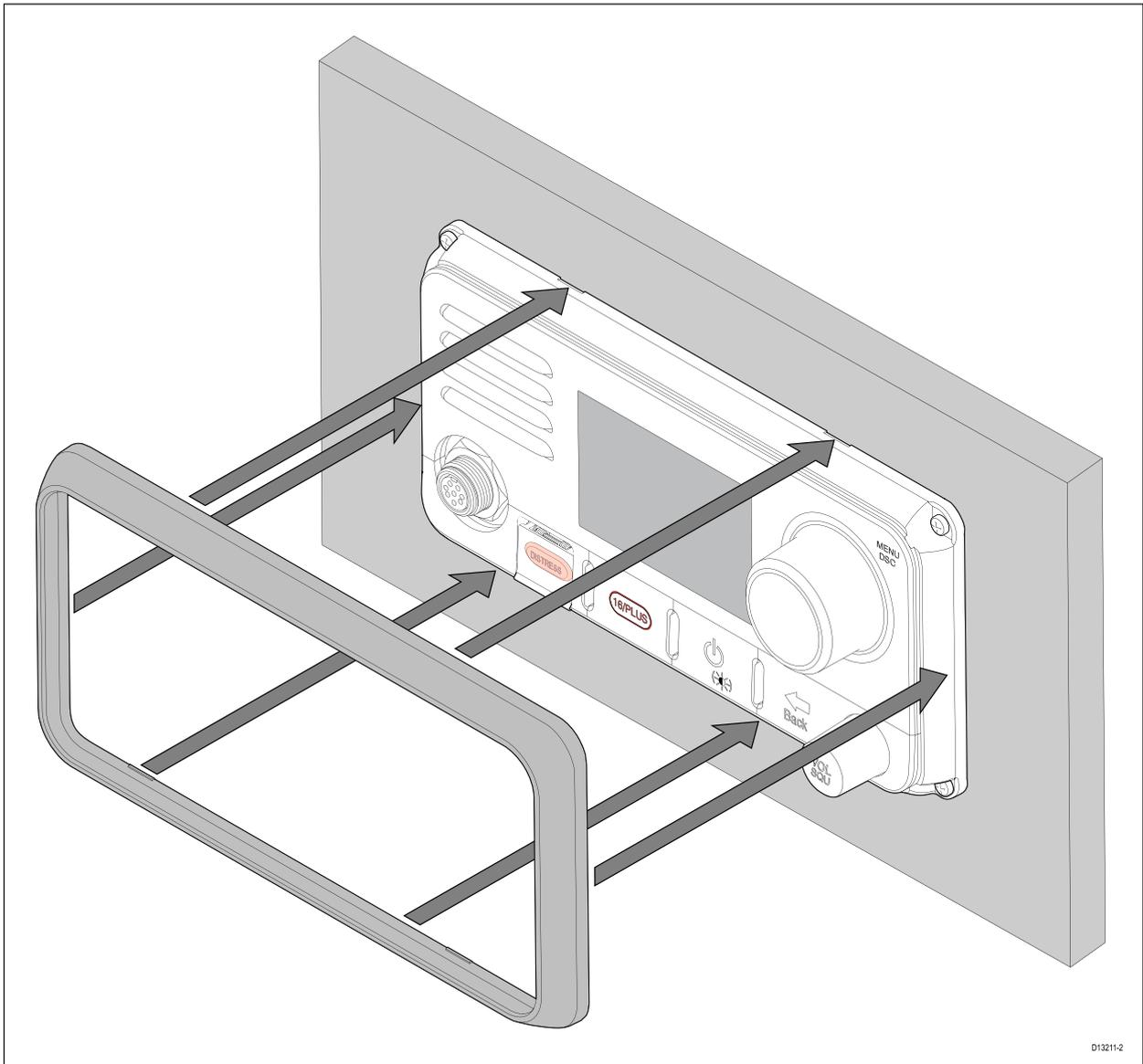
2. Ensure the bezel is correctly aligned with the unit, as shown.
