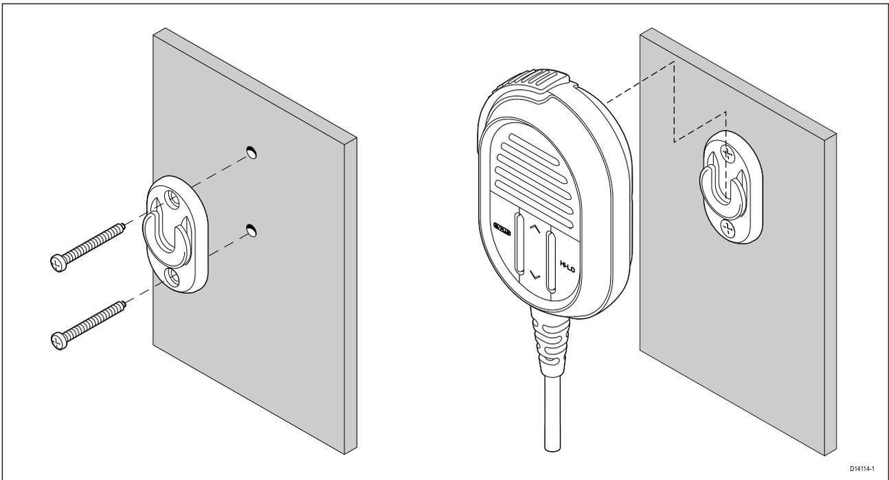
1. Check the selected location for the Hook plate, a clear flat area is required, with sufficient space around it to place and remove the Fistmic / Handset and coiled cable.
