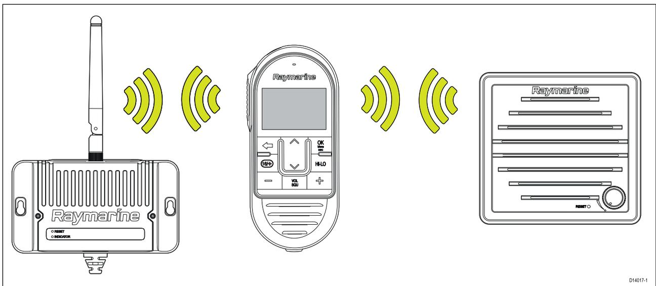
Up to 2 Wireless handsets can be connected to the Wireless hub. Refer to [6.2 Connecting a wireless handset to the hub](#) for the connection procedure.
