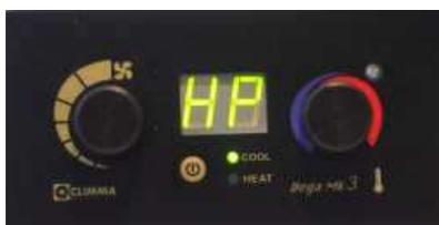
System locked by safety cut out (HP)
