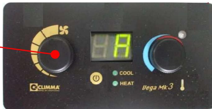
**Important note:** if the functioning mode AF- Auto-special is selected, the fan speed range is automatically limited. In COOL mode the minimum speed is #5 in auto and #3 in manual. In heat mode the minimum speed is #3. In heat mode, if the HP safety stops the compressor, at restart the speed is rised by 2 steps both at first and at the second intervention. At third intervention the system is locked out.
