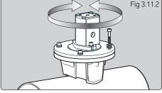
Motor ports require male/female connectors with correct size hydraulic sealing washers.
