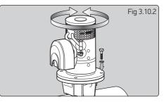
Remove drive shaft key retaining tie, grease shaft, slide motor into position and align holes for most suitable installation and bolt motor assembly to saddle applying Blue Loctite<sup>®</sup> 243 to bolts.
