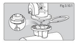
Coupling is factory fitted. DO NOT remove.
