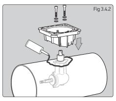
NOTE: Poor exterior tunnel surface could cause leakage and noise. Apply sealant to this area as required (Fig. 3.4.2).
