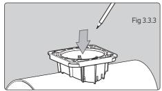
Place the thruster saddle in the desired position, ensure the fit is firm and free from movement then mark centre.
