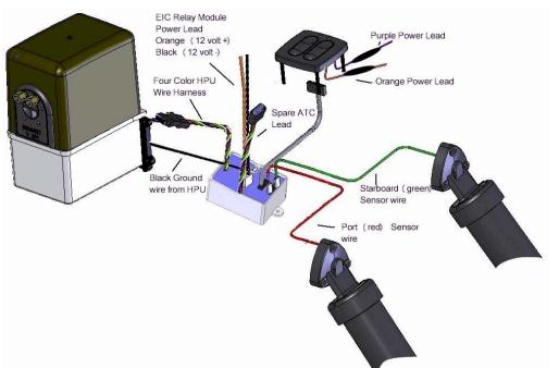
HPU Connection: Plug the 4-color wire harness from the Hydraulic Power Unit into the Hydraulic Power Unit Wire Harness (longer of the two harnesses) on the Relay Module.
