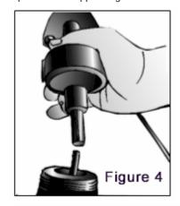
hinge onto cylinder while keeping metal rod inserted into center of sensor coil (see figure 4). Red cable for port side and green cable for starboard side. Tighten upper hinge hand tight.
